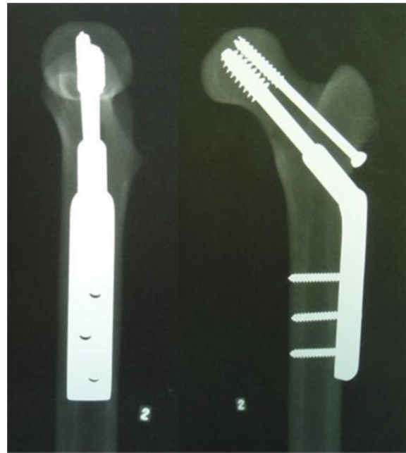
Fig. 2 – Radiograph on synthetic bone fixed with DHS before the test.
