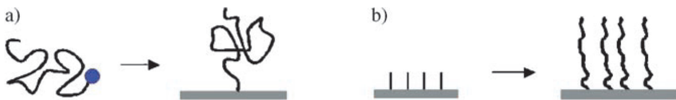
Figure 1. Chemisorbed polymers prepared by a) graft-to, or b) graft-from approach.
