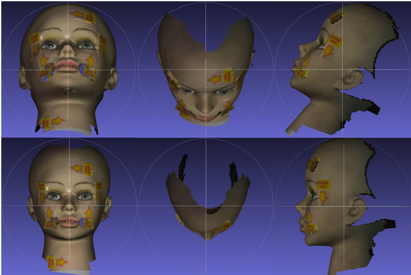
Fig 6. Validation of the automatic orientation method on a plastic head. The alignment laser was placed at the center of SP device (which was perpendicular to the NHP mirror) and were indicated with the arrow stickers. Top row: frontal, top and left lateral views of reconstructed facial surface from 3dMD. Bottom row: corrected surfaces with the proposed method.
