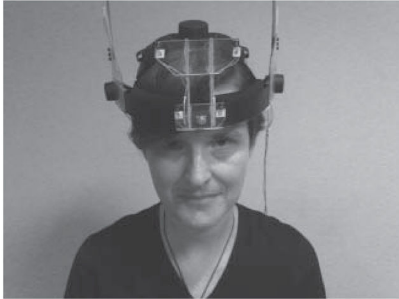
Figure 9. The head device that holds the light-emitting Optotrak markers.
