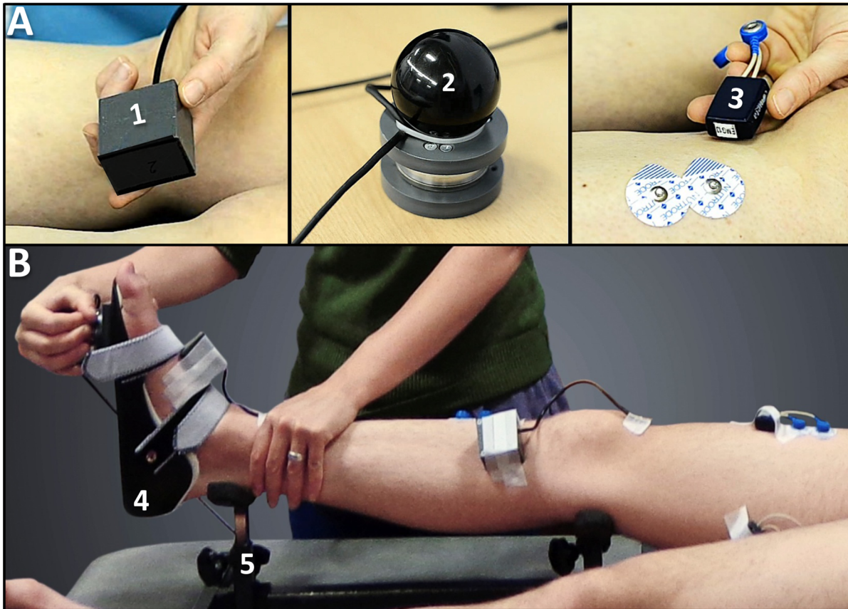
Fig 1. A. Measurement instrumentation. (1) three inertial measurement units (joint angle measurement); (2) a six degrees of freedom force/torque-sensor (torque measurement); (3) surface electromyography (muscle activation measurement); B. Measurement set-up for assessing the lateral gastrocnemius. (4) custom ankle orthosis; and (5) support frame. [25].
