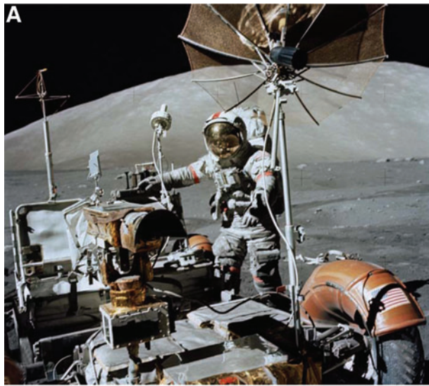
FIG. 7. Crewed extravehicular activity (EVA) vehicles for planetary explorations. (A) Apollo 17 astronaut Eugene Cernan during third EVA at Taurus-Littrow standing adjacent to the unpressurized Lunar Rover (NASA image AS17-134-20476). (B) NASA's Space Exploration Vehicle (SEV) configured here as a small pressurized rover during field testing at the Black Point Lava Flow site, Arizona. (C) EVA suits mounted on suit ports on the rear bulkhead of the SEV. Color images are available at www.liebertonline.com/ast .
