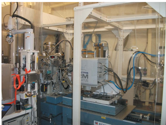
Figure 4 A photograph of the long-wavelength beamline BL-1A at the Photon Factory (courtesy of Naohiro Matsugaki). The beamline has been optimized for data collection using X-rays in the range from 2.7 to 3.5 \text{\AA} , with the entire experimental station enclosed in a helium box to reduce air absorption at longer wavelengths.
