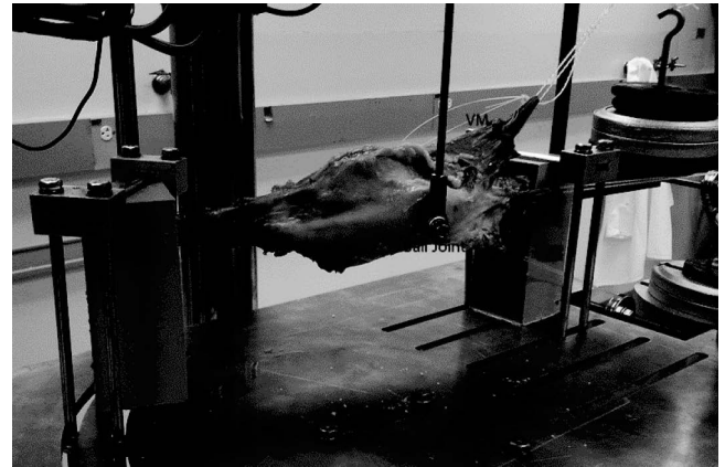
Figure 3. Experimental setup with the knee mounted in the Bionix II material testing machine with the quadriceps loaded using a custom pulley system through the cloth loops.
