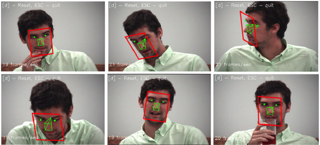
Fig. 2. Examples of head tracking during moderate to large head motion and occlusion. The examples are from Sayette Group Formation Task data set [53].
