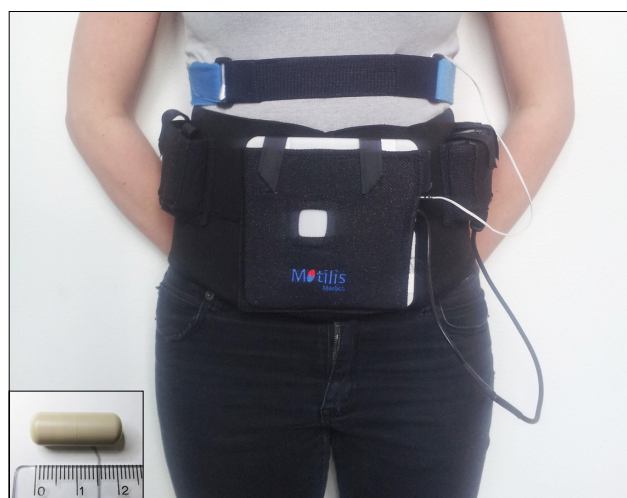
Figure 1. 3D-Transit system. Electromagnetic signals from the ingestible capsule (inset) are registered by sensors in the detector plate. The detector plate and its battery are worn in an abdominal belt. A respiration belt is placed above the detector to remove respiration artefacts. Data are stored on a SD card in the detector.
