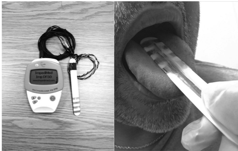
FIGURE 1. The ImpediMed DF50 and tongue probe equipped with four-electrode array used to measure EIM measures (left). The typical probe placement at the midline of the tongue (right).
