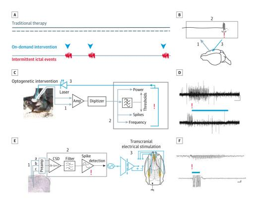
Figure. Closed-Loop Intervention to Inhibit Spontaneous Seizures
