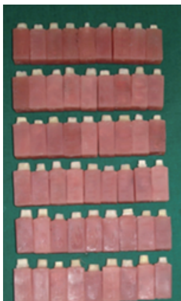
Figure 2. Prepared teeth mounted vertically in auto polymerizing acrylic resin.
