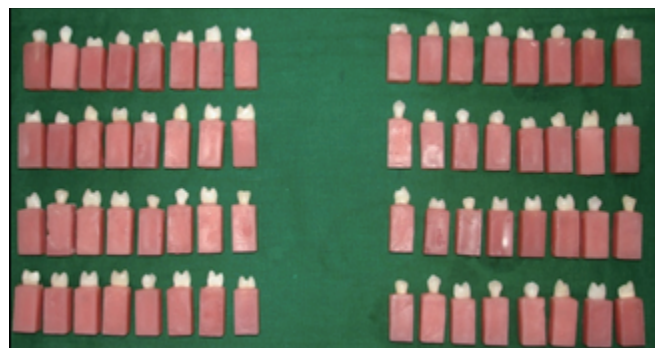
Figure 1. The teeth are mounted vertically in auto polymerizing acrylic resin.
