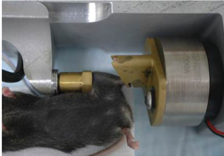
Figure 4. Mouse situated in loading device, ready for in vivo axial loading to be applied to the left tibia.
