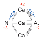
Figure 14. Bond graph for the metallic perovskite AuNCa_3 , in which summing bond orders (in blue) of N and Ca, obtained from 8– N and 8 + N rules, respectively, yields an invalid oxidation state for Au.
