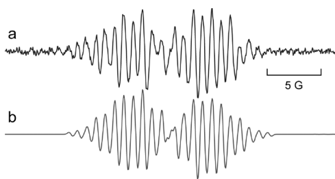
Figure 4. EPR spectra from photolysis of acid 4d in PhH at 300 K. a) Experimental spectrum from 4d . b) Computer simulation.
