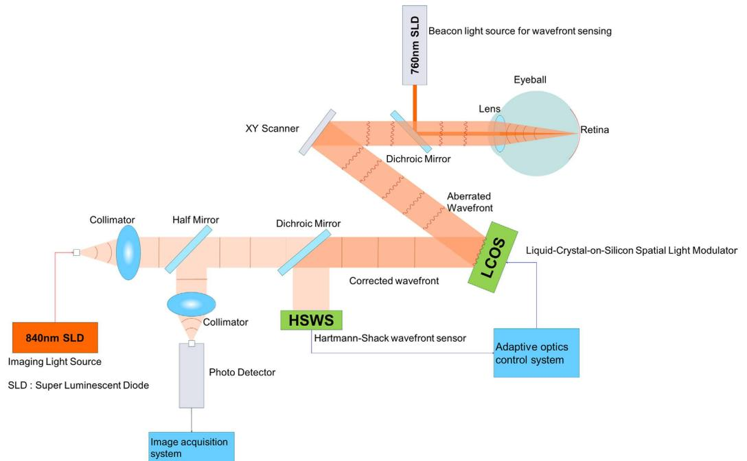
**Figure 4. Schematic of adaptive optics scanning laser ophthalmoscopy.** A spatial light modulator, based on the Liquid-Crystal-on-Silicon, and a wavefront sensor, based on the Shack-Hartmann sensor, was used to compensate for wavefront errors. The high-resolution imaging system was a confocal scanning laser ophthalmoscopy with light emitted from an 840-nm superluminescent diode.
