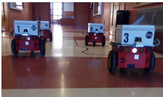
Figure 6. Experimental test using four P3-DX robotic units remotely controlled by a personal computer.
