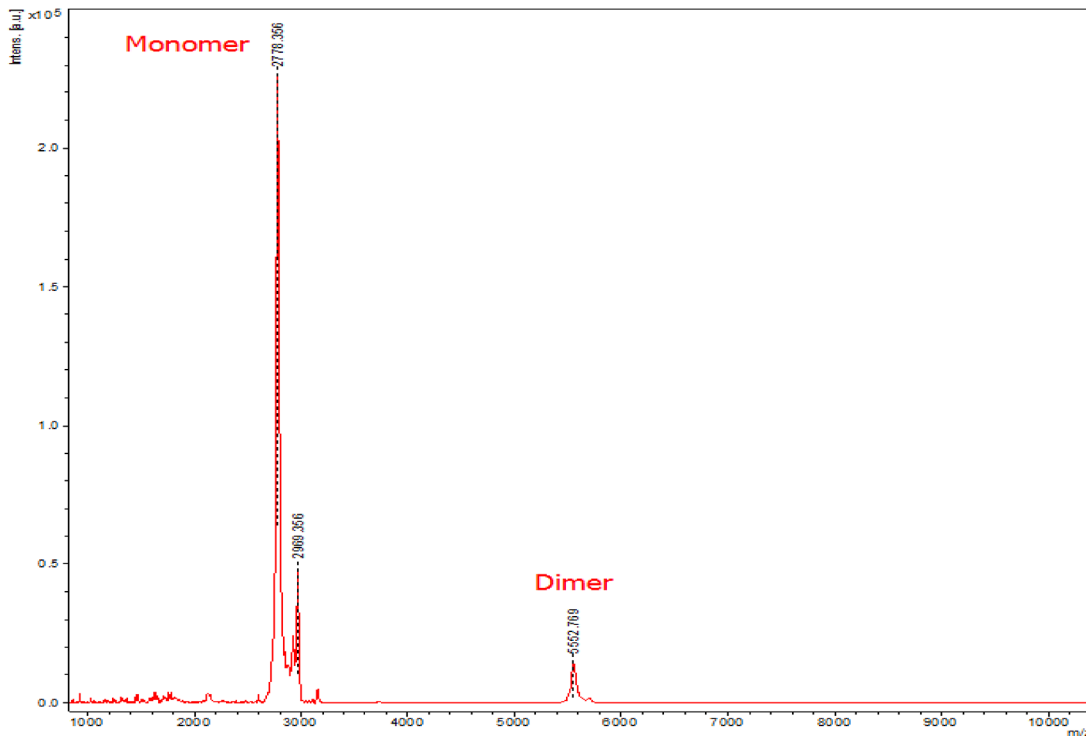
Fig 4. Linear mode MALDI-TOF mass spectrometry analysis of PA-dPEG24 oligomeric state. PA-dPEG24 in acidified water was analyzed by linear mode mass spectrometry. The spectrum shows two peaks for PA-dPEG24 with a monomer peak at 2778 and a dimer form at 5553.
