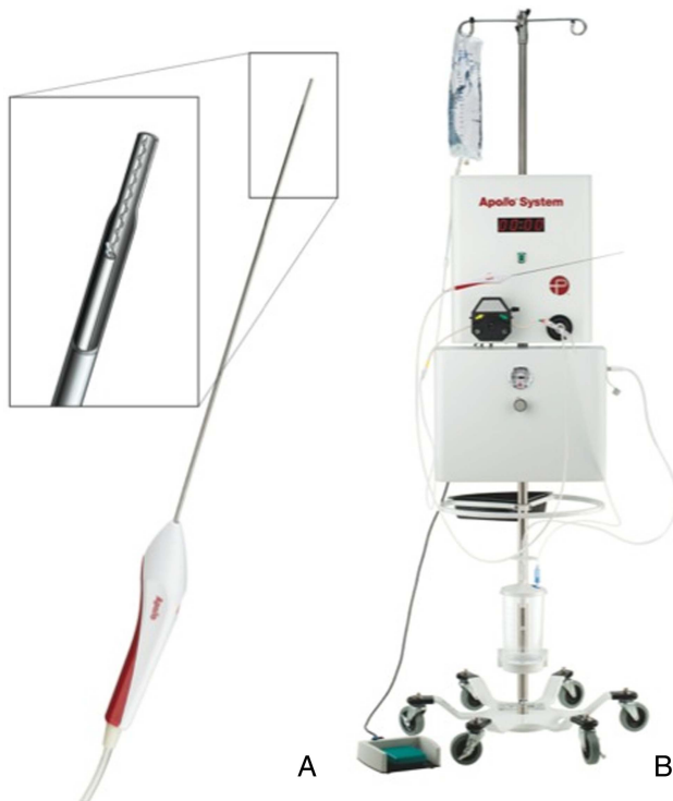
Figure 1 The Apollo system is composed of an aspiration–irrigation system, which can be attached via flexible tubing to the Apollo wand. The wand (A) can be accommodated by an 8F vascular sheath. The 2.6 mm wand houses an internal agitator wire that macerates clot material to maintain patency of the system during aspiration. The wand is attached to the freestanding aspiration–irrigation system (B). The aspiration–irrigation system (B) provides the capability for aspiration and saline irrigation and transmits vibrational energy to the internal agitator element within the wand.
