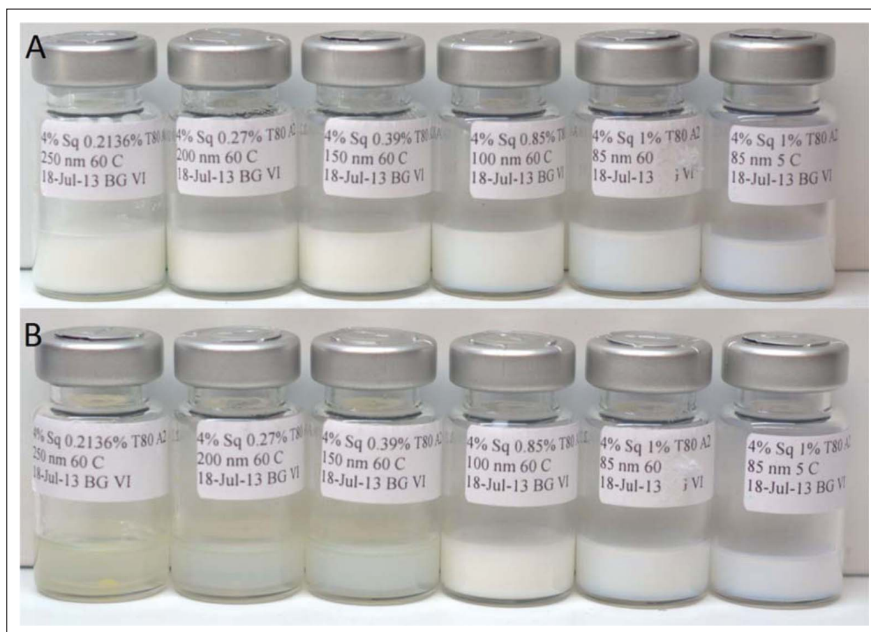
Figure 4. Pictures of the emulsion reveal phase separation of the emulsion when stored at 60°C for up to 2 weeks (A) and one month (B). No phase separation was observed in the 80 nm emulsion particles as observed in samples with particle size of 150 nm or higher.
