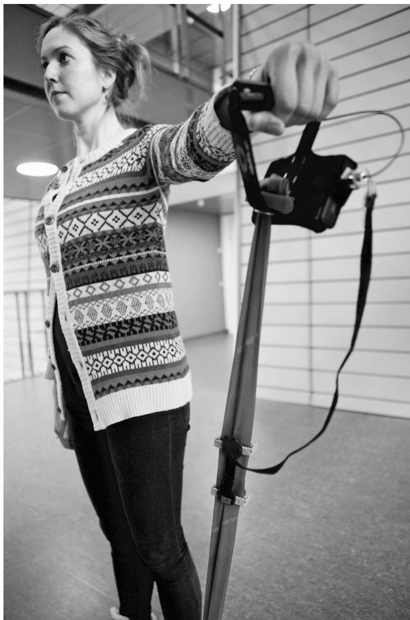
Figure 1 Shoulder abduction with the stretch-sensor attached to the elastic band.
