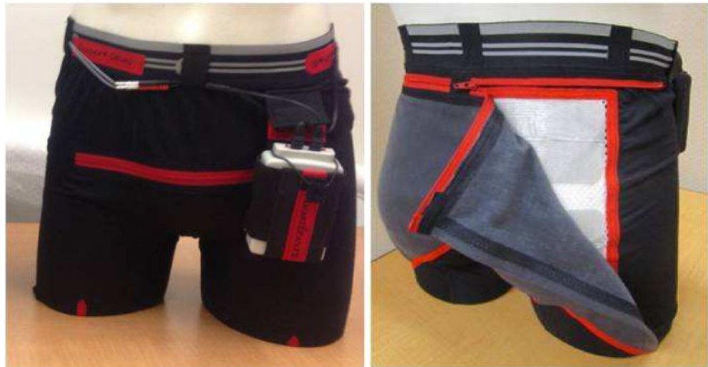
Figure 9. “Smart-e-pants” system showing garment, mesh panel for surface electrodes and stimulator.
