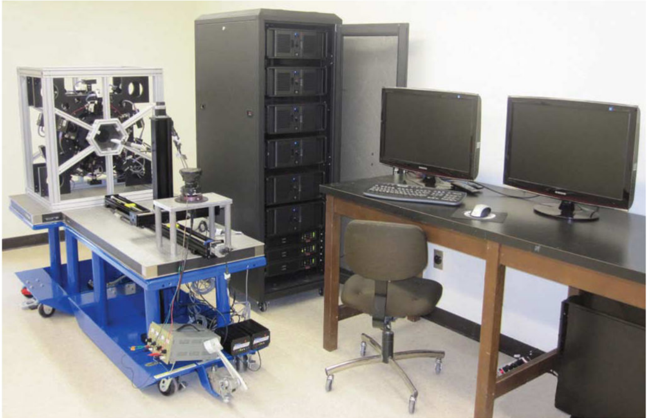
Fig. 1. FastSPECT III stationary SPECT imaging system. The system comprises 20 BazookaSPECT detectors and acquisition hardware that processes \sim 1.23 Gpix/s. In the current imaging configuration, the detectors share a common FOV of \sim 15 mm for neurological imaging studies of the mouse brain.
