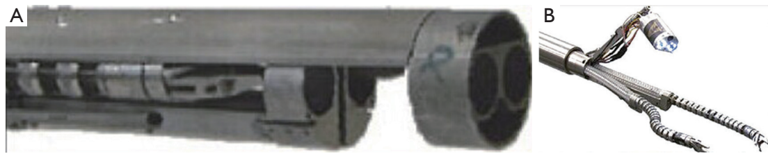
Figure 16 A new insertable robotic end-effectors platform (IREP, Columbia University, USA) (17). (A) The cylindrical profile with the diameter of only 15 mm before opened up; (B) the robot opens up with camera and arms when it is inserted into the thoracic cavity.
