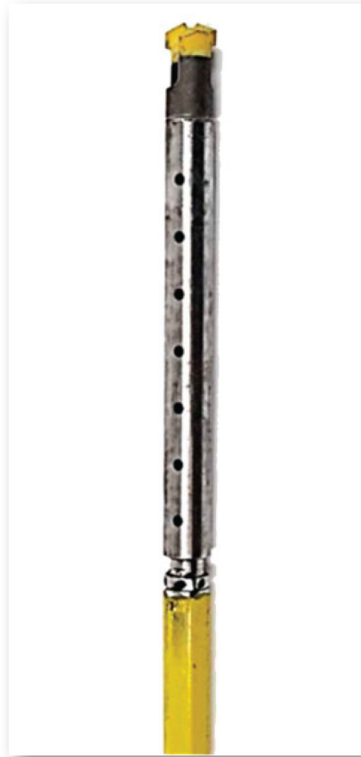
Figure 2. Drill bit isolator installed with 35-mm (1.3-in.) drill bit and hexagonal drill steel.
