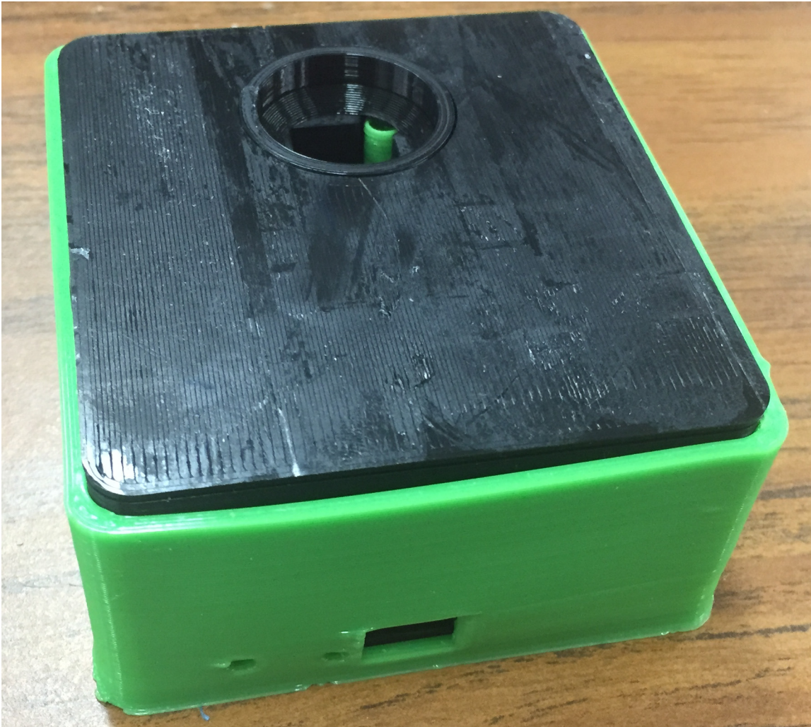
Fig 6. Photometer case with TPE protective outer case.
