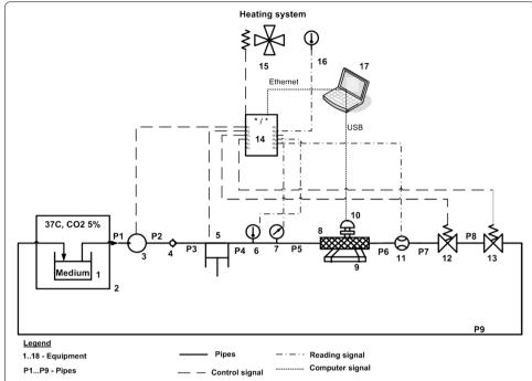
**Fig. 4** The in vitro test bench. The different parts of the in vitro test bench are depicted. *1* reservoir, *2* incubator, *3* centrifugal pump, *4* one—way valve, *5* custom designed piston pump, *6* thermocouple, *7* pressure sensor, *8* test section, *9* microscope, *10* CCD camera, *11* flow meter, *12*, *13* solenoid proportional valves, *14* AC/DC controller, *15* heating system, *16* thermocouple, *17* PC class computer/notebook/touch screen computer.
