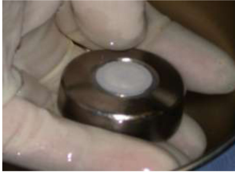
Figure 1. Oxygen sensor array with integrated wireless telemetry system at implantation. The electrodes are imbedded into a ceramic disc that is hermetically sealed into the titanium housing. The electrodes are covered by a PDMS membrane. The implant is 3.4 cm in diameter and 1.5 cm thick.
