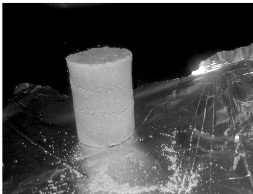
Fig 9. Raw propolis sample obtained after supercritical extraction using CO 2 and ethanol as co-solvent.
