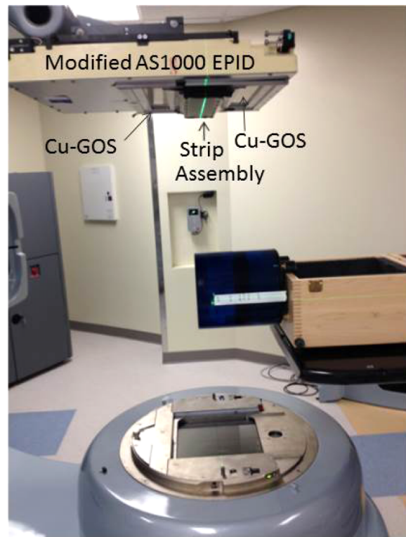
FIG. 7. Modified AS1000EPID mounted to a Varian Trilogy Clinac. The top cover of the strip assembly, which traverses the entire width of the imager, is visible. In the surrounding portions, the EPID is coupled to a Cu-GOS scintillator. The CatPhan phantom, hanging off the front edge of the patient able, is also visible.
