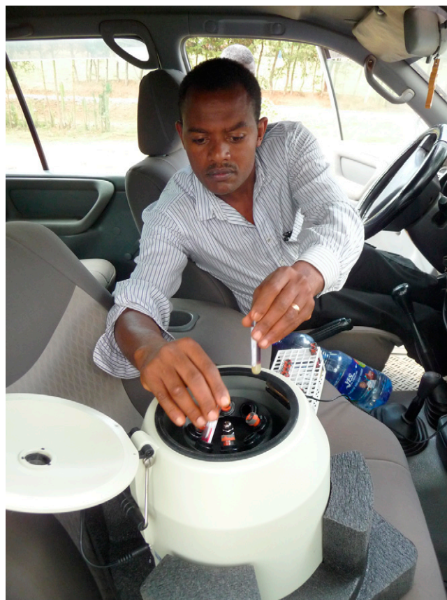
FIGURE 4. Serum samples were centrifuged on-site within 4 hours using a portable centrifuge (Portafuge ™ ) that plugged into the field vehicle.
