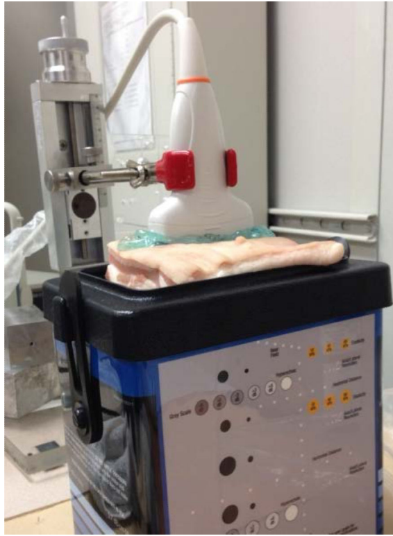
Figure 8. Experiment setup with a piece of excised pork belly in between the transducer and the phantom.
