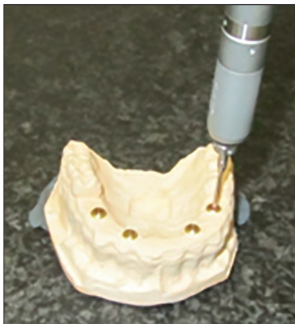
Figure 3: The coordinate measuring machine probe measuring the relative distances of analogues.
