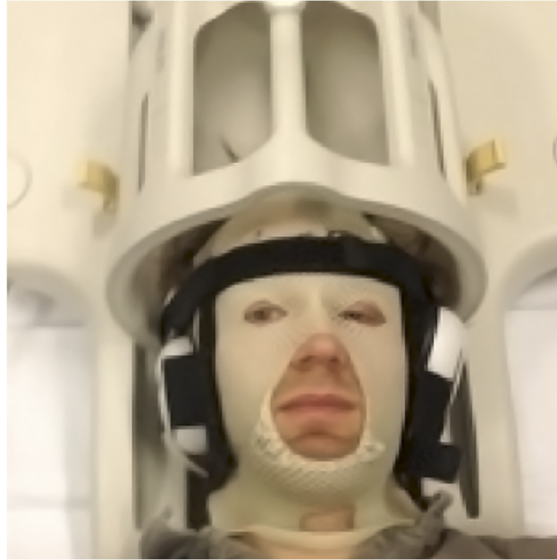
Fig 3. Head immobilization set-up, with a subject strapped to the coil using individual thermoplastic mold and three Velcro attachments.
