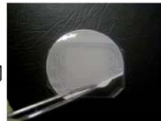
b: (Left) The functionalized membrane and activated PDMS microdevice are brought into contact. (Right) A picture of the bonded laminate.
