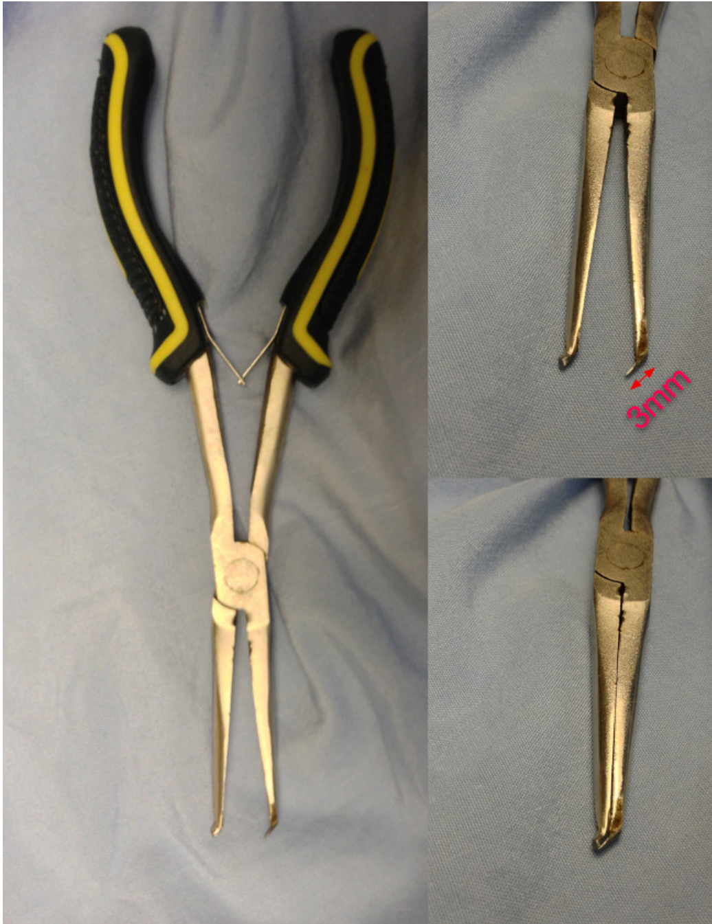
Figure 1. The custom-made bone cutter for laminectomies. The thin blade is designed to slide beneath the lamina. Please click here to view a larger version of this figure.
