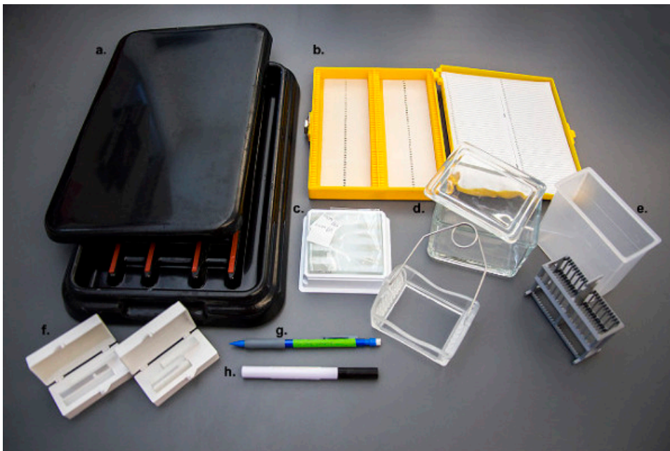
Figure 3: Example items required for immunohistochemical staining. The black box shown in (A) is an ideal humidity chamber for immunofluorescence, as slides are protected from light without the need to wrap the box on foil. Following sectioning, slides can be stored in a box such as the yellow box shown in (B). Wrapping the box tightly in foil and placing in a zip-top bag prior to the freezer helps protect the tissue samples from freezer burn. An example of slides is given in (C), with different staining dishes depicted in (D) and (E). Coverslips can vary in size and thickness (F), however 1.2 thick coverslips provide nice imaging results on most upright and confocal microscopes. A pencil such as that shown in (G) can be used to label slides. Permanent markers should be avoided as the ink can run, affecting both staining and the ability to determine what the sample is. A mini pap pen such as that shown in (H) enables a repellent border to be drawn on slides.
