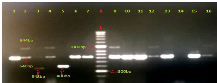
Fig. 1 Result of Multiplex PCR of GBS isolates resistant to erythromycin and clindamycin. Lane 8 DNA Molecular Weight Marker Hyper Ladder™ 50 bp (BioLine). Lane 14 negative control (GBS ATCC 49447). Lane 1, 6, 7, 10, 11, 13, 15 presence of ermB genes, 640 bp, (sample no 15, 63, 65, 125, 148, 182, 183). Lane 2, 4, 9, 12, 16 presence of both ermB genes and linB genes, 944 bp (sample no 32, 57, 191, 159, 184). Lane 5 presence of ermTR gene, 400 bp (sample no 83). Lane 3 presence of mefA gene, 348 bp (sample no 60)
