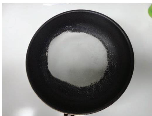
Figure 1 The coating of the centre of the pan was burned off.
