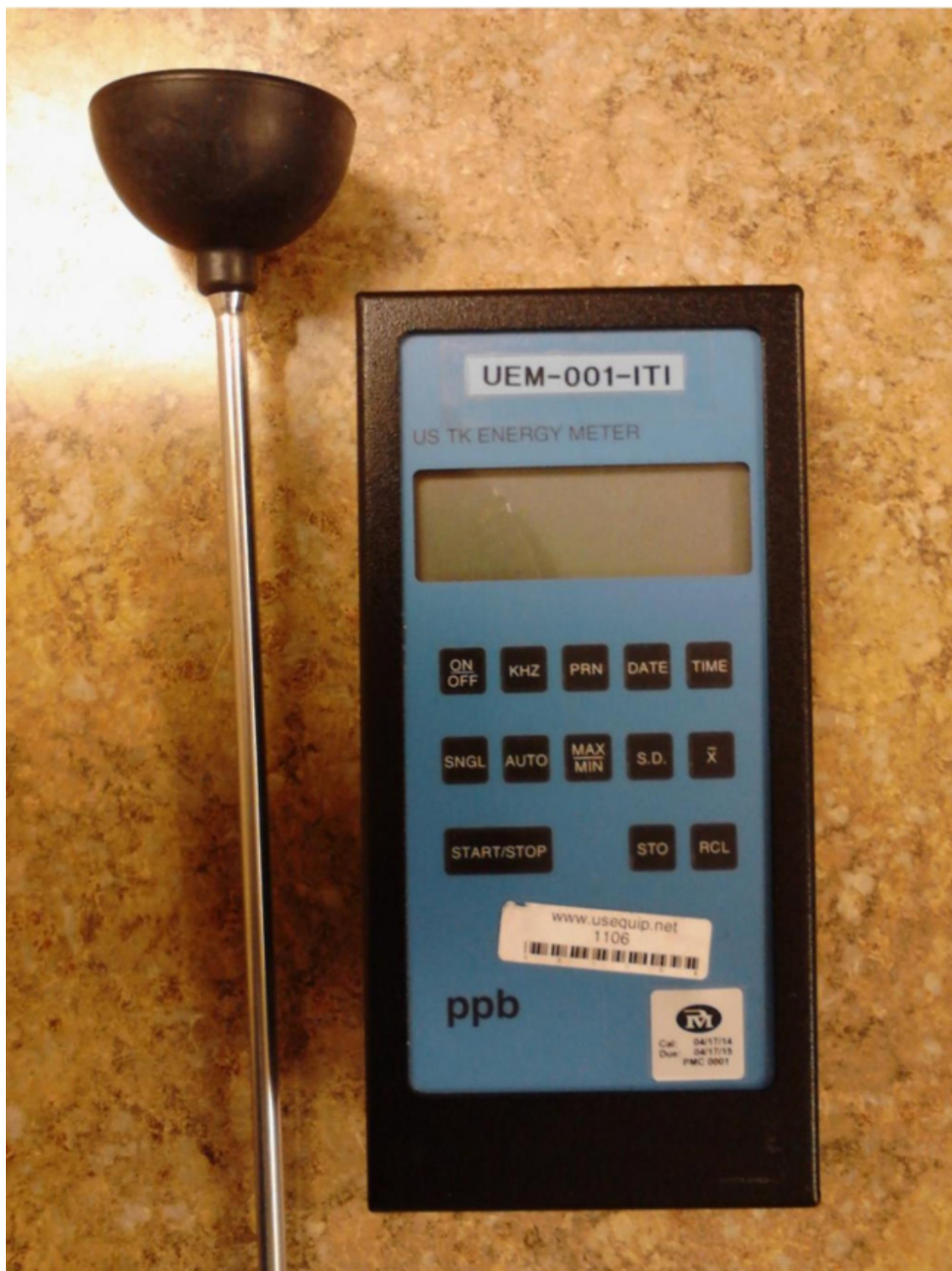
Figure 4. Use of a cavitation meter to characterize the sound intensity of the ultrasonic system. The cavitation meter seen here is used to represent cavitation energy in W/cm^2 . This is a very important instrument for assessing consistency of energy with respect to the sample.
