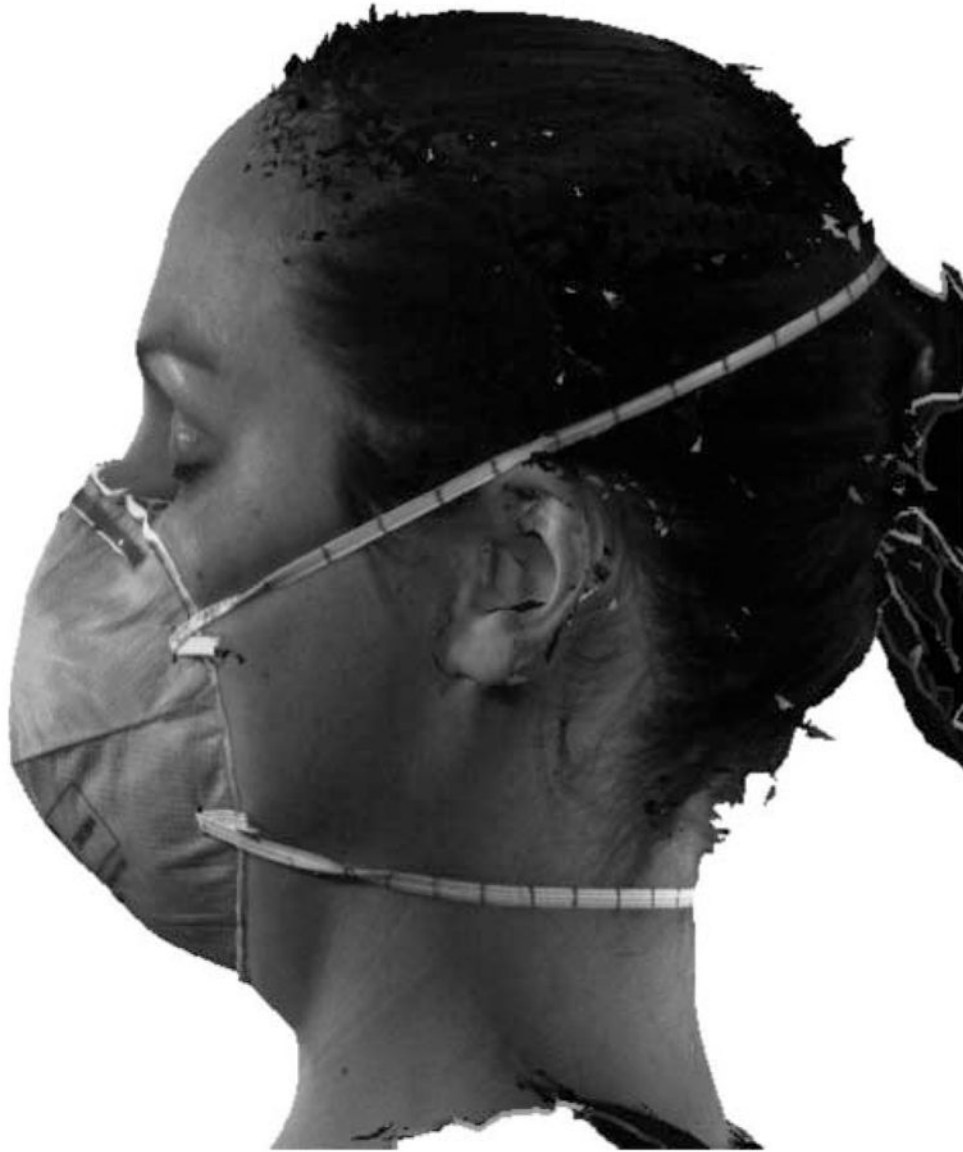
FIGURE 1. N95 filtering facepiece respirator with 1-cm gradations marked on the tethering devices for use in determining stress and strain for pressure calculations.
