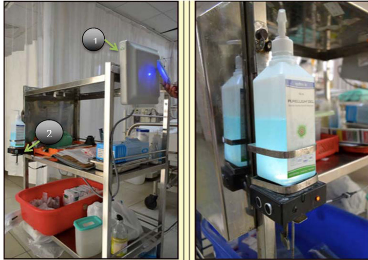
Fig. 1. Fig 1(a) Patient trolley with the RFID reader (1) and sanitizer module (2) Fig 1(b) Close-up of the hand sanitizer module with the glowing LED
