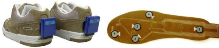
Figure 1. SmartShoe device: (left) Overall view of the shoe device with attached accelerometer, battery and power switch on the back; (right) Pressure-sensitive insole with 5 pressure sensors: heel (1), 3rd metatarsal head (2), 1st metatarsal head (3), 5th metatarsal head (4), hallux (5).
