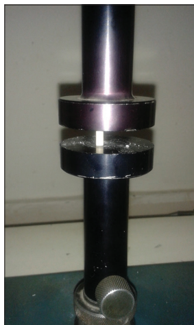
Figure 5: Specimen being tested for compressive strength using Universal Testing Machine
