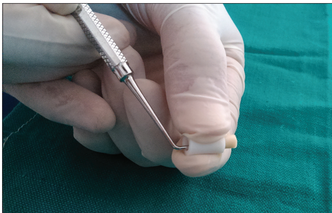
Figure 1: Specimens allowed to set at room temperature and teased out of molds
