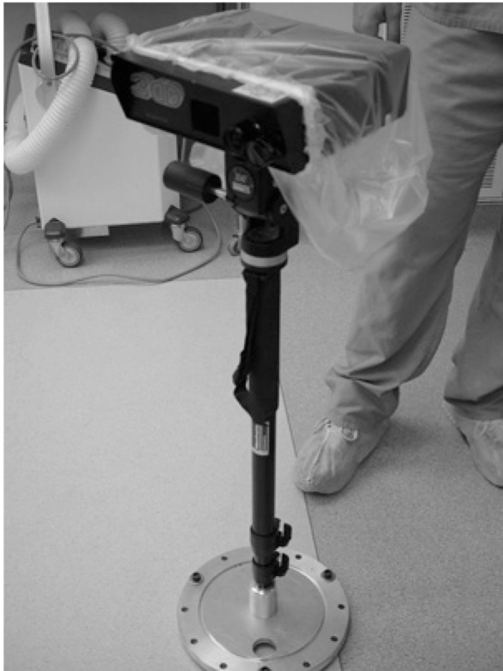
Fig. 1. Laser range scanner mounted on vibration damping monopod in OR.
