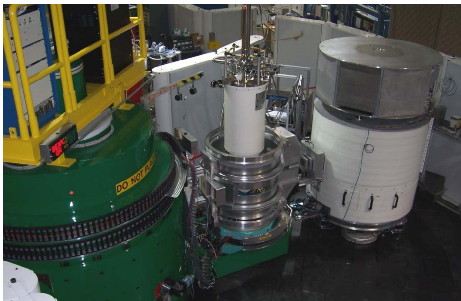
Fig. 4. Photograph of the thermal triple axis instrument at BT-7 in operation. The electronics for the front portion of the instrument (through the sample position) resides on top of the (green) monochromator drum, while the sample environment system is the top-loading He 3 system with a base temperature of 300 mK. The sample is surrounded by the sample enclosure to adsorb scattered neutrons and reduce ambient instrumental background. The analyzer system is below 17^\circ so that the beam stop is in the up position. Two PG filters and an x-y slit system are on the x-rail in front of the analyzer system. The electronics for the analyzer system resides on top of the analyzer.
