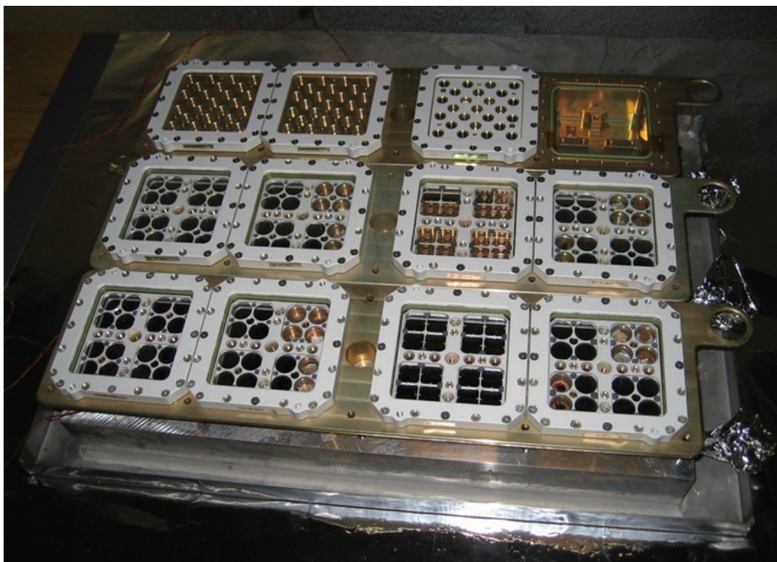
FIG. 1. Experimental setup of the simulation procedure at the Microgravity User Support Center (MUSC) at DLR Cologne utilizing the EXPOSE-E/-R hardware for ground-based Scientific Verification Tests (SVT). The samples in tray 1 (front row) were exposed to vacuum of 4.1 \times 10^{-5} Pa, those in tray 2 (middle row) to Mars atmosphere and pressure (780–930 Pa). Additionally, the upper layer was irradiated with a total UVR 200–400nm fluence of 5.7 \times 10^5 kJ m -2 , and the samples were subdued to irradiation-dependent temperature cycling temperatures between -25^\circ\text{C} in the dark (16 h) and +10^\circ\text{C} during irradiation (8 h). (Color images available at www.liebertonline.com/ast )
