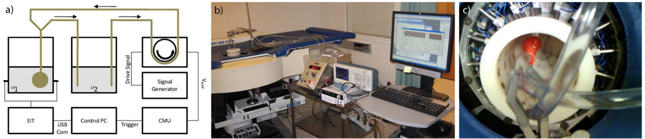
Fig. 2. Phantom dynamic imaging experimental configuration. a) Schematic representation of interconnected electrical and fluid systems, b) physical configuration, c) balloon position within saline tank.
