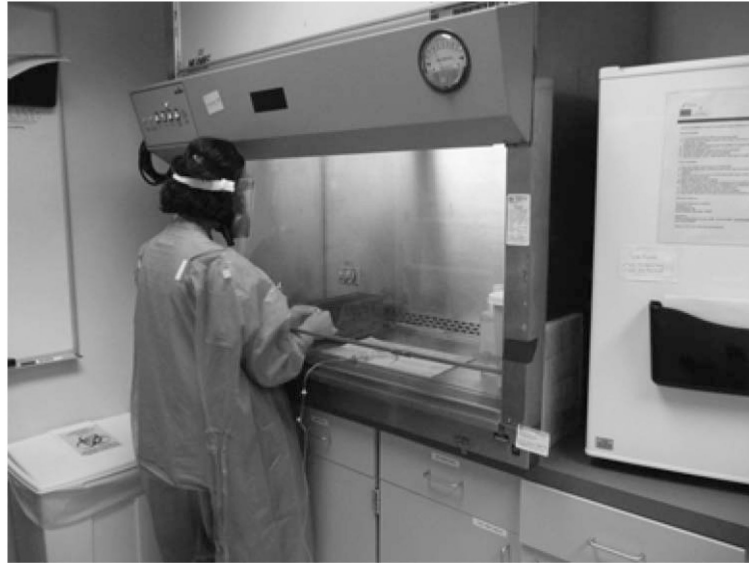
FIGURE 1. Veterinary technician wearing personal protective equipment while preparing chemotherapy drugs in a Class II biosafety cabinet.
